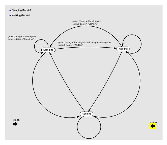
Notice that the above FSM provides direct transitions between each of the states, even between **Stopped** and **Running**. This means that the application should be able to classify two subsequent variances as belonging to each of these states, and does not require a pass through the **Walking** state.
